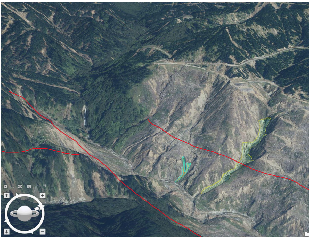
Figure 5: Absence of buffer below topographic break in slope (red lines) where it is most needed.
