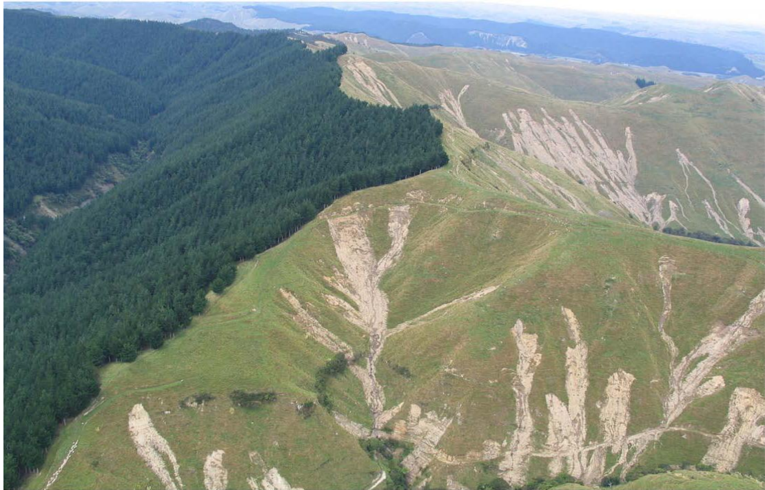
Figure 1. Effectiveness of a closed-canopy forest in preventing landslide initiation compared with similarly steep but treeless pastoral land within terrain classed as highly susceptible to the initiation of shallow landslides and where due to the absence of plantings the probability of sediment reaching a stream channel is also high, that is, high connectivity.
