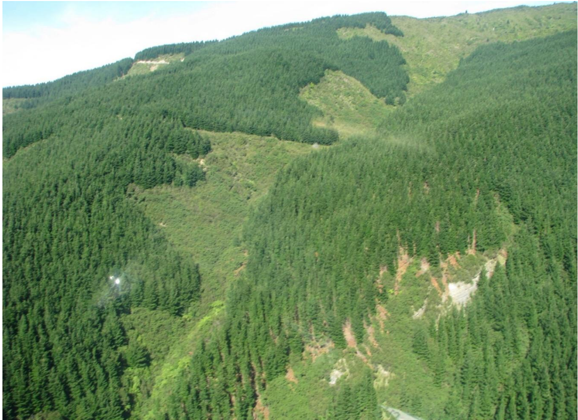
Figure 2: An example of a buffer planned and implemented before forest establishment and with the foresight of providing a sufficiently extensive buffer that at the time when pines are harvested would intercept slash and sediment before it reached the channel (likely an ephemeral stream).
